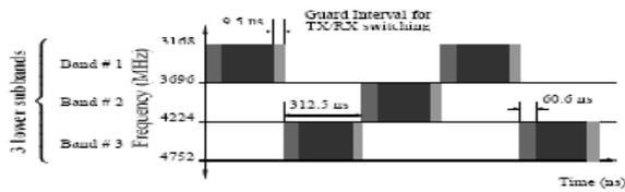
Fig. 3. Example of Time-Frequency Code in MB-OFDM system.
